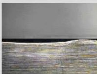
従来型（固定）ガイド使用の刃物摩耗拡大写真 When the conventional type (fixed) guide is used. A closeup picture of the blade worn out
